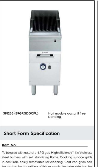
in cast iron, easily removable for cleaning. Cast iron grids can be rotated for the grilling of fish or meats. Includes drip tray for the collection of grease and fat. Exterior panels of unit in stainless steel with Scotch Brite finish. Extra strength work top in heavy duty 2 mm stainless steel. Rght-angled side edges to allow flushfitting junction between units.
